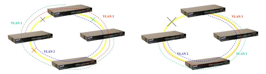
MSTP – balance bandwidth for each link since each VLAN have its own spanning tree instance
